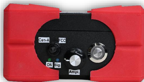
Device side view with G3PLC band switch, amplitude level knob and on-off switch
